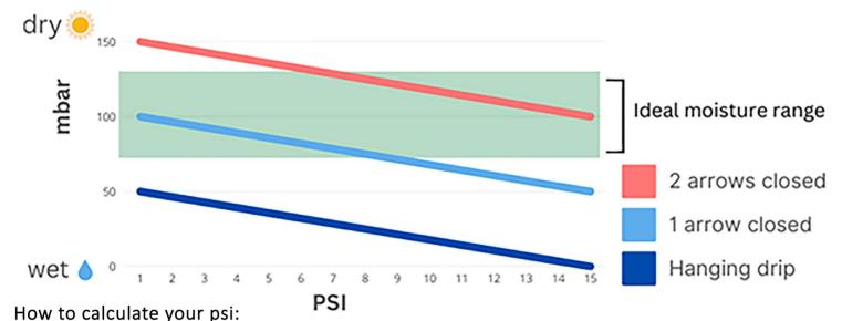
Measure from the top of the water line of your reservoir to the soil surface in feet and divide by 2.31
